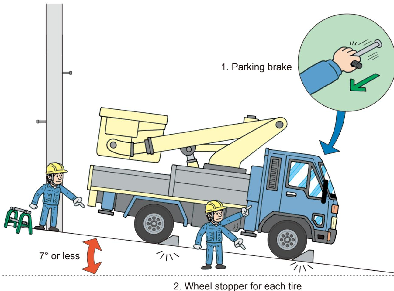
1. Be sure to park the vehicle on a slope with the front part low, apply the parking brake securely, and check that the vehicle does not move even if the foot brake is released.
