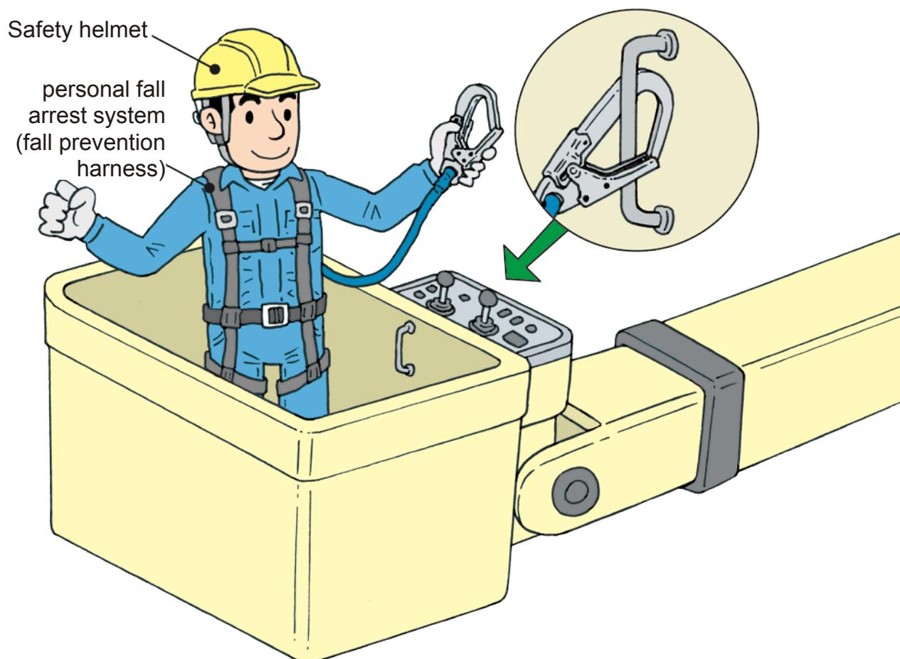
1. A passenger in the bucket must wear the proper personal fall arrest systems.
