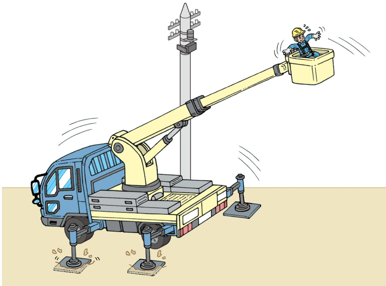
1. If you work on a soft ground with road shoulders or contains plenty of water, be careful because the jack under heavy load may sink and fall.
