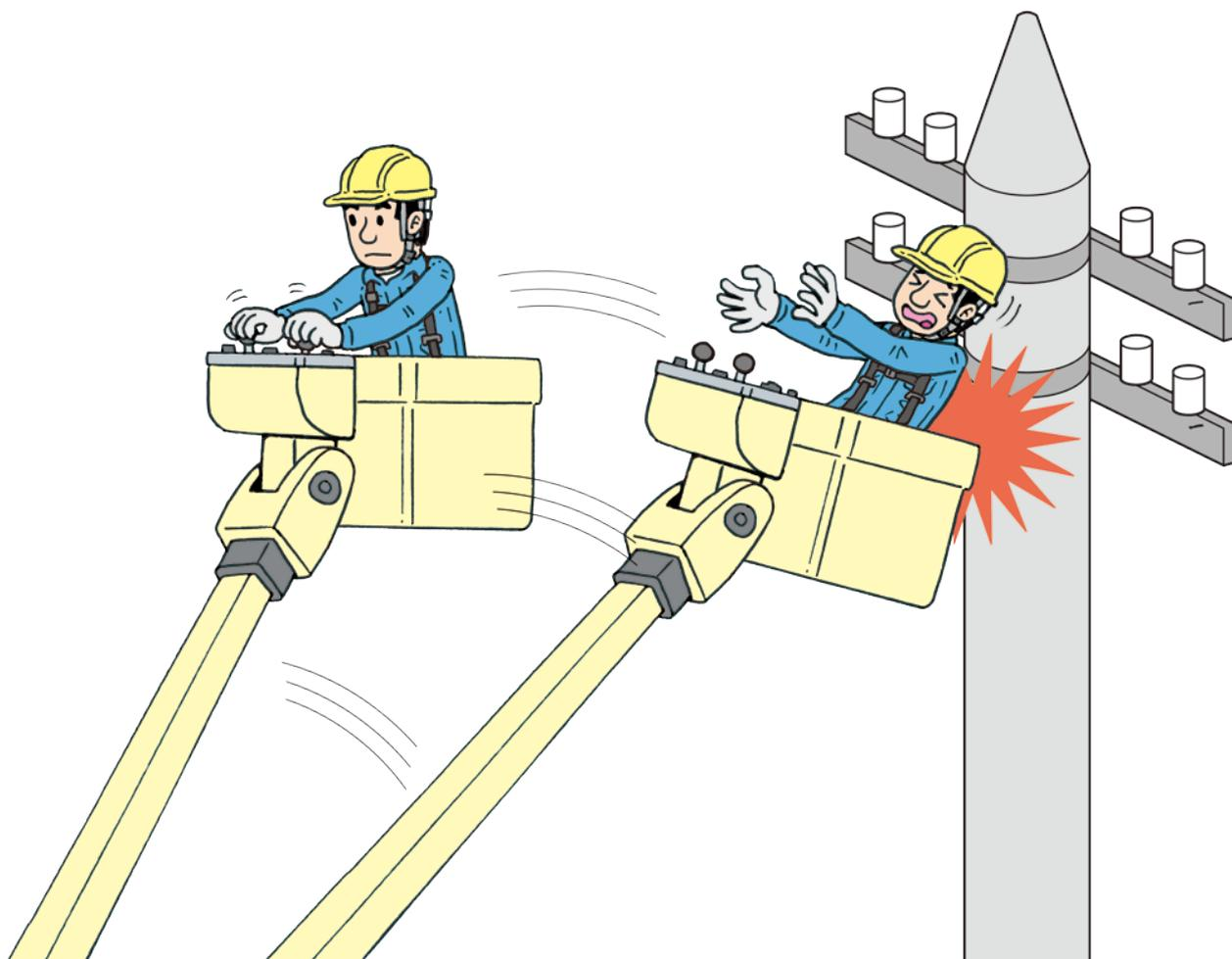
Revolving and derricking operations move faster and the impact increases when a boom is extended. For turning and derricking operations near the work position, switch the accelerator to lower speed, and operate the lever one by one, or position the bucket with telescopic or swinging operation.
