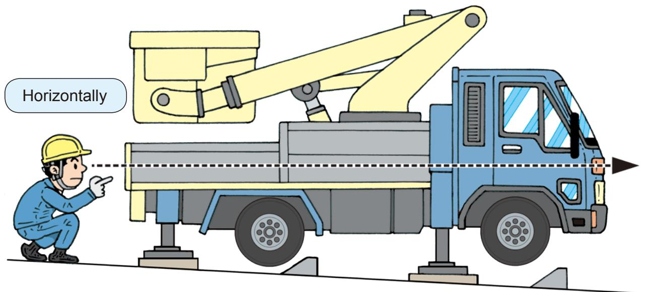
1. Regardless of the slope of the road, jack up the vehicle until it is horizontally leveled.
