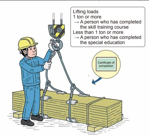
\*"**Lifting loads**" is not the weight of the lifted loads, but the lifting loads of a crane or a mobile crane used.
