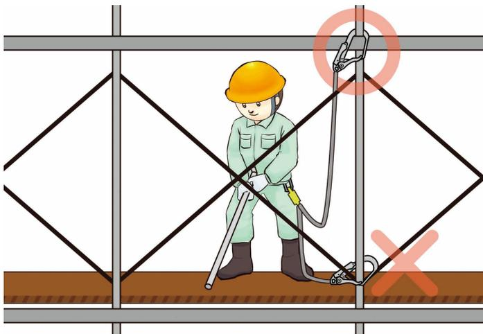
**A worker will suffer a fracture due to impact when dropped.**
